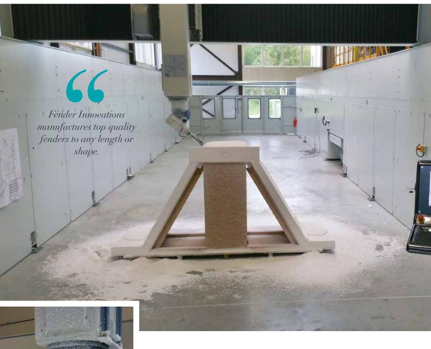
that is of remarkable low weight when compared to other fenders on the market. Their fenders are built with a cross-linked PE foam core making them up to twelve times lighter than traditional rubber fenders. The seamless corners and customised fit give the fenders a sleek design and also improve protection, dampening, and wear and tear characteristics.
